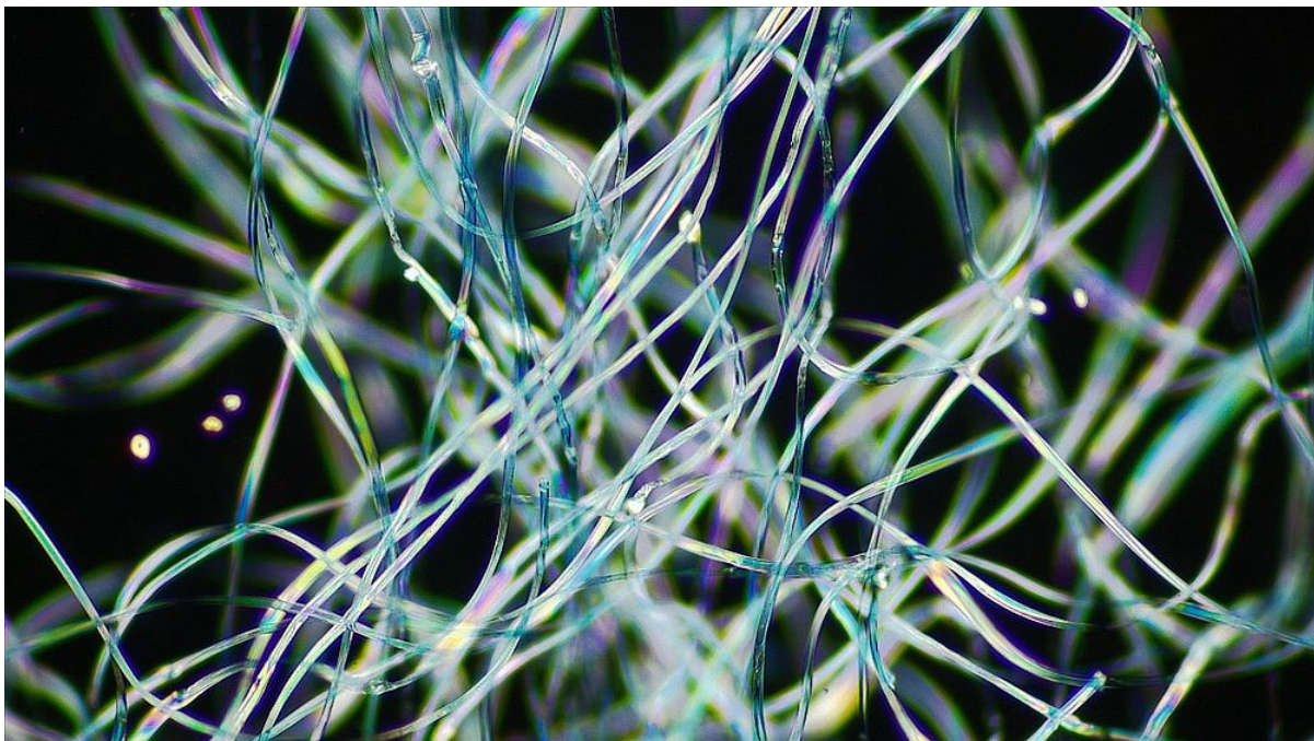
Polyester fleece fibres pictured under a microscope
