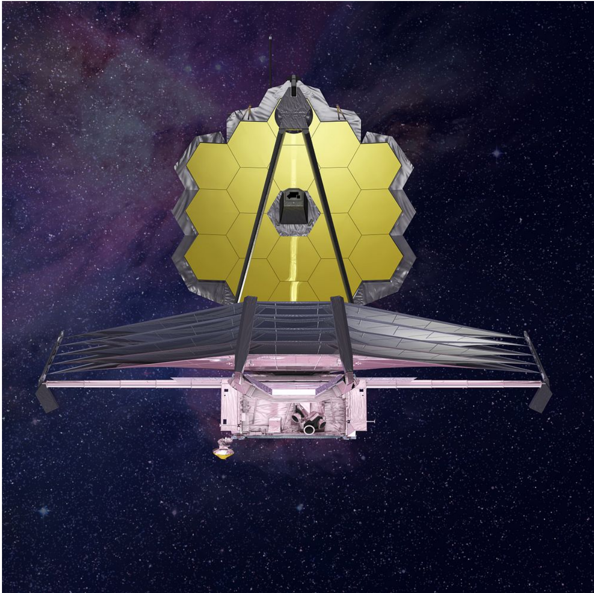
An illustration of the Webb telescope showing the segmented mirror and layered sunshield. Image credit: NASA, ESA, CSA, Northrop Grumman
